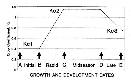
Figure 1. Generalized crop coefficient curve for field crops
