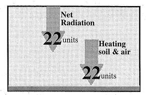
For simplicity, energy units are not shown. The size of and number on arrows represents accurate proportions of incoming and outgoing energy under irrigated grass and bare soil conditions.
