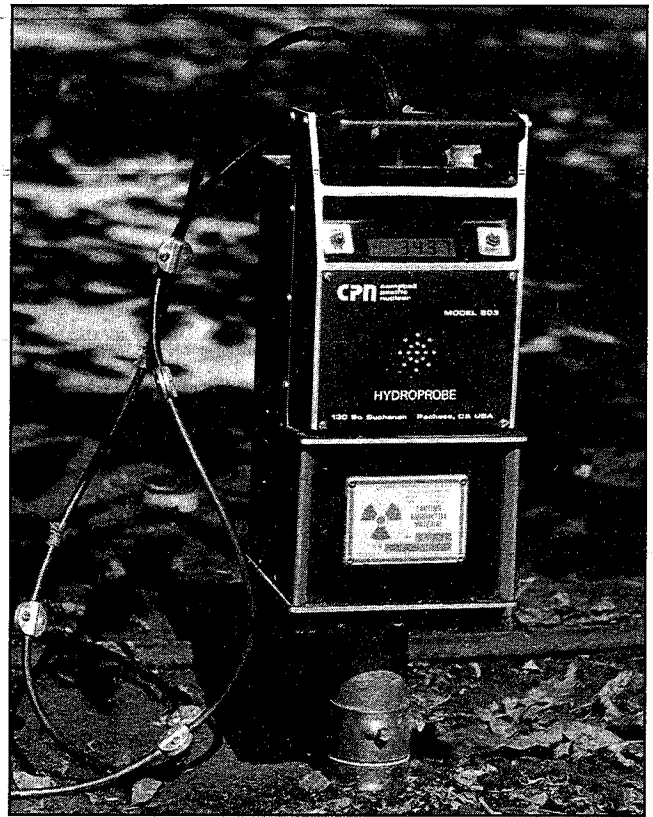
Neutron probe measurements show the water distribution in the soil profile.
